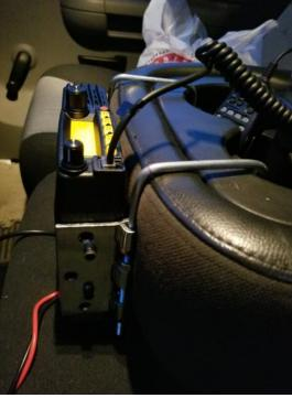
points under the dashboard to keep the coax away from my feet while driving. REMEMBER: You want nothing between you and the pedals when driving. A stray piece of wire or coax could prevent you from applying the brake or gas properly and possibly cause an accident. Once inside, I attached a PL-259 connector to the coax end.
